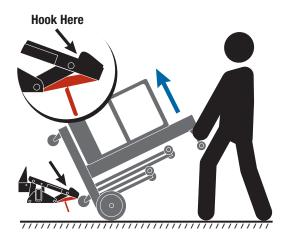
With the PowerLift "hooked" over the Rocker Plate Glides, lower the PowerLift on to the Rocker Plate (Figure 3-8).
