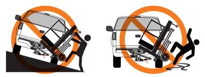
Figure 1-4: Do not load or unload on uneven or slippery surfaces
