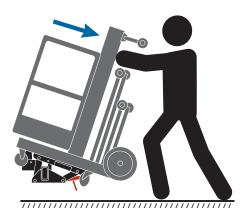
**4.** With the Rocker Plate down, continue to tilt back the PowerLift to the ground, unhooking from the Hitch Hauler (**Figure 3-15**).
