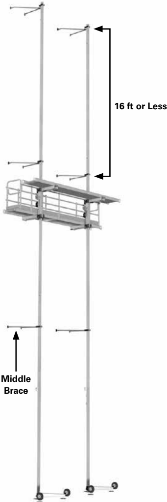
Figure 6.6 - Supporting the Mast
