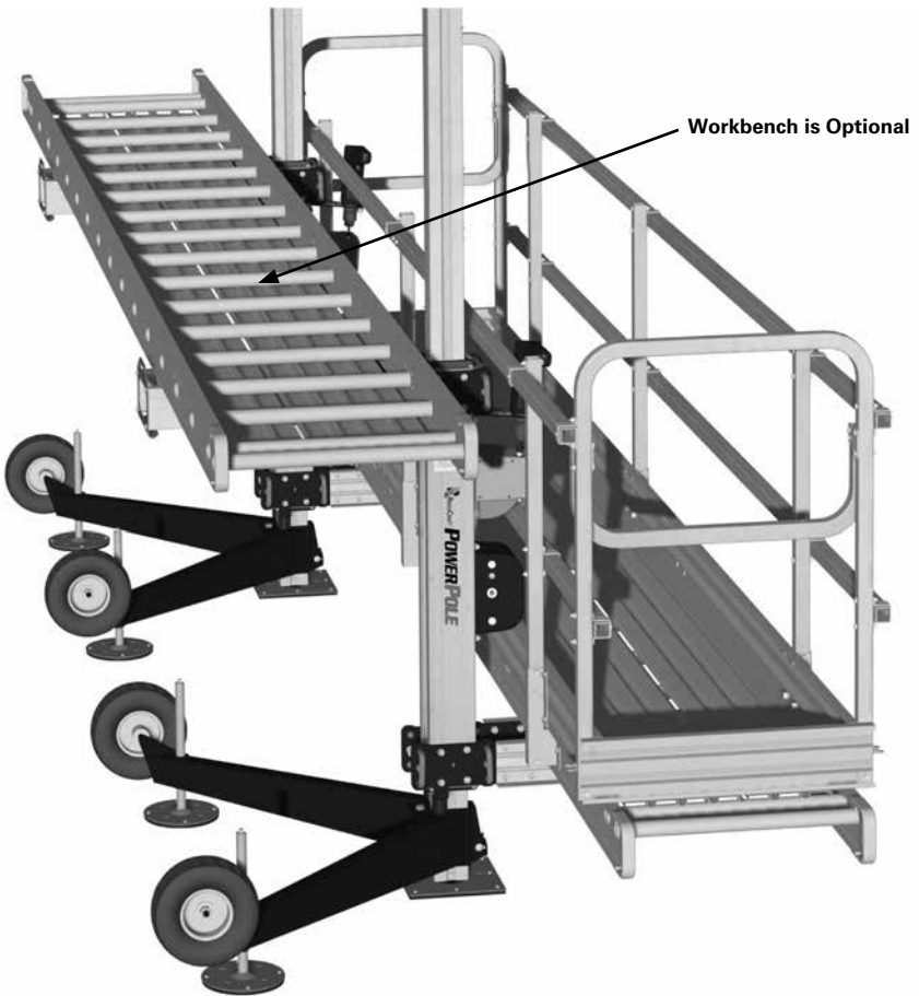
Figure 4.3 - Work Bench Installation
