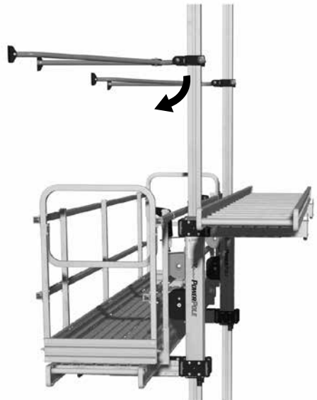
Figure 6.7 - Disconnecting the Tie
