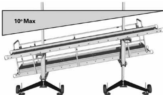
Figure 6.3 - Leveling the Platform
