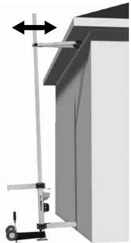
Figure 3.11 - Equalizing the Mast Assembly
