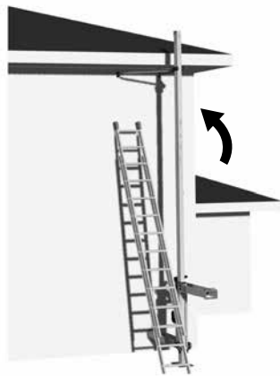
Figure 3.1 - Lifting the Assembly (2 of 2)
